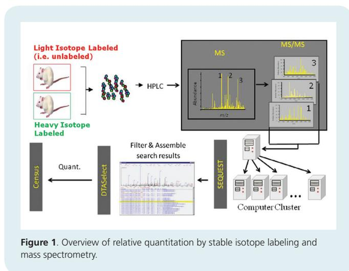
**Figure 1.** Overview of relative quantitation by stable isotope labeling and mass spectrometry.
